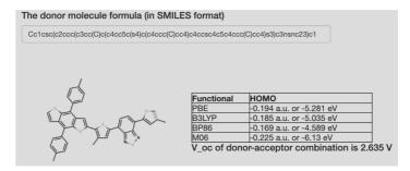
**FIGURE 13** Screenshot of the the web application with response illustrating the molecular compound of the SMILES input with the predicted HOMO values across 4 functionals: PBE, B3LYP, BP86 and M06
