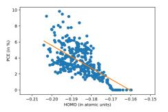
**FIGURE 2** The scatter-plot (with line of best fit) demonstrates the linear relationship between PCE of the device and HOMO values of the donor compound. The boltzmann average of the HOMO values for each conformer is used to determine the HOMO for a given donor.
