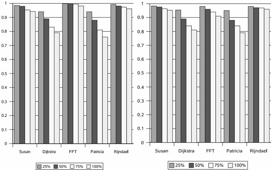
**Fig. 3.** Performance as a function of encryption of varying basic block lengths before(left side) and after(right side) performing loop unrolling on the benchmarks. (25%, 50%, 75% and 100% basic blocks are encrypted)
