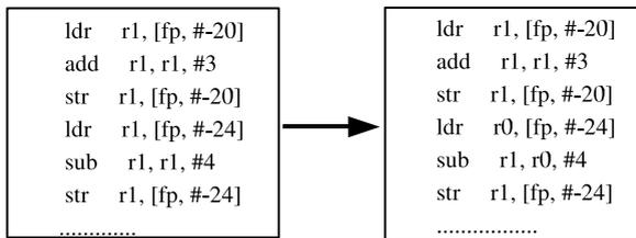
Fig. 2. Register encoding example with key 11010000011
