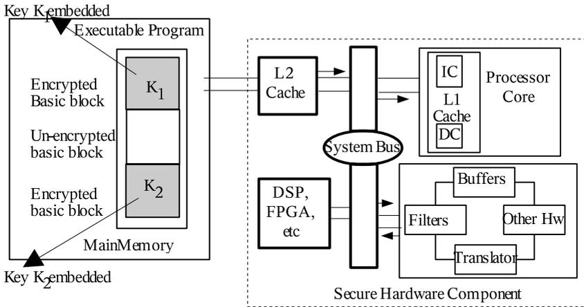
Fig. 1. System architecture
