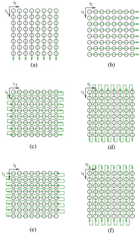
**Figure 1:** (a-b) Access directions along  $i_1$  and  $i_2$  loops. (c-d) Two different access patterns depending on the nesting order of the loops. (e-f) Access patterns in the opposite direction of (c-d).
